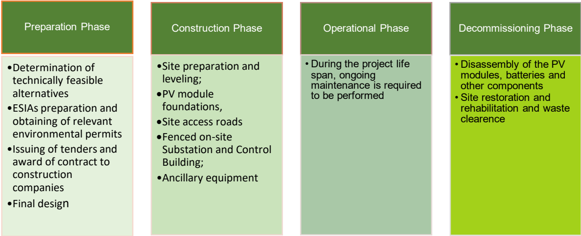
Figure 5: General Stages of PV Project Construction
